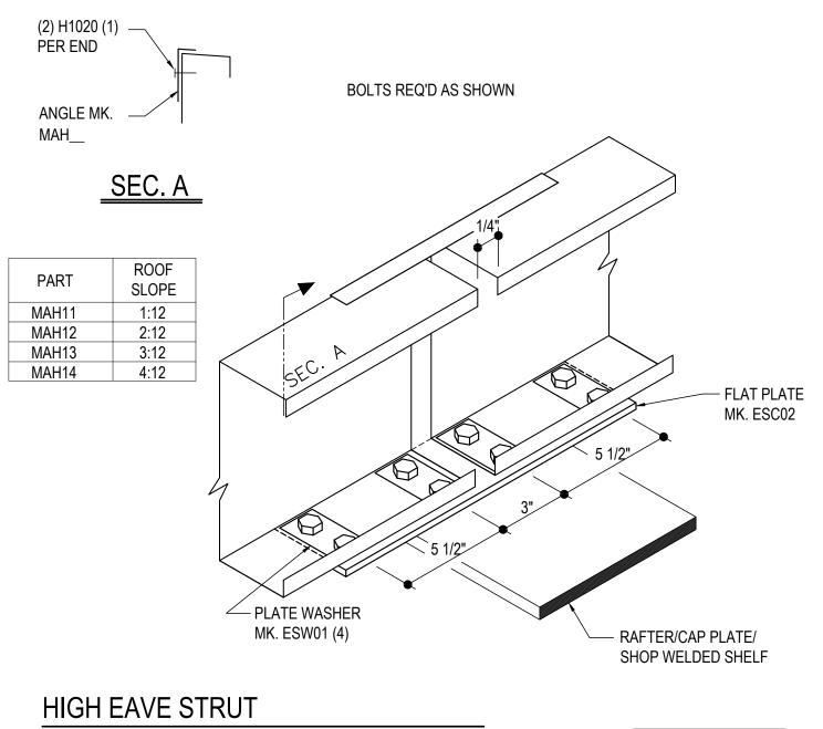
HIGH EAVE BYPASS SW GIRT CONDITION WITH STRUT PLATE USE (8) 1/2" X 2" A325 BOLT H0603/NUT H0300 U.N.O.
