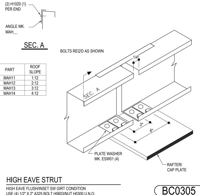
HIGH EAVE FLUSH/INSET SW GIRT CONDITION USE (4) 1/2" X 2" A325 BOLT H0603/NUT H0300 U.N.O.
